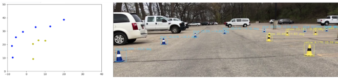
Fig. 4. YOLOV3 Model Finding Yellow and Blue Cones using the ZED stereo camera
